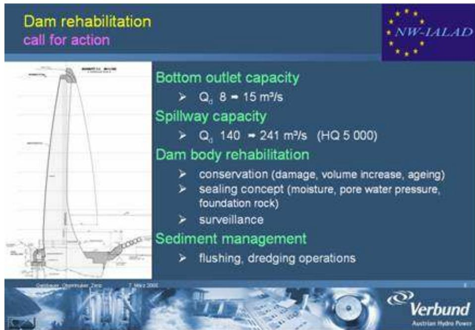
*Figure 3: Factors to be considered during refurbishment*
